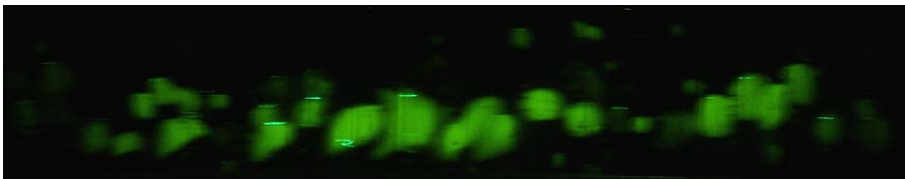
Fig. 6. Dispersed flow pattern in the 5.6 mm pipe. Mixture velocity U_{\text{Mixture}} = 1.94 m/s, input water volume fraction \hat{\epsilon}_{\text{Water}} = 0.105 , Reynolds number of the mixture Re_{\text{Mixture}} = 9'095 .
