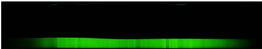
Fig. 3. Stratified flow pattern in the 5.6 mm pipe. Mixture velocity U_{\text{Mixture}} = 0.70 m/s, input water volume fraction \dot{\epsilon}_{\text{Water}} = 0.291 , Reynolds number of the mixture Re_{\text{Mixture}} = 3'410 .
